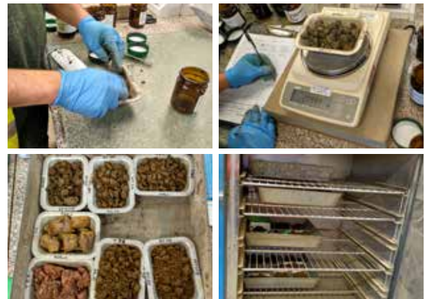
Figure 5. Top left to right – weighing trays and describing samples, laboratory report. Bottom left to right – trays with soil samples ready for oven drying, trays in the oven.
