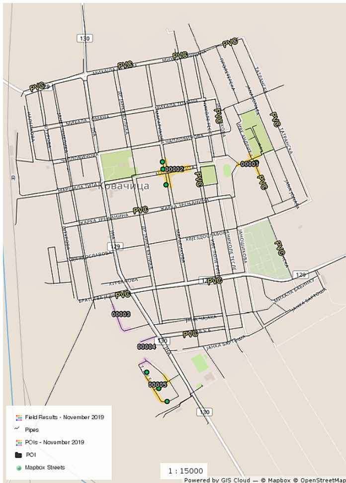
Figure 7. Water supply network of Kovačica settlement with locations of detected (and potential) leakage
