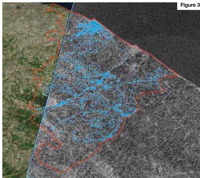
Utilis-supplied data of pipeline routes are used in conjunction with the satellite imagery (Figure 3) to indicate points of interest (POIs) that are likely leak locations (Figure 4). Images supplied by 2F Water Venture
